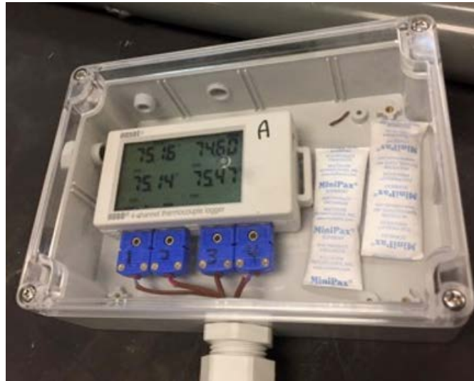
Figure A.3: Data logger housing
